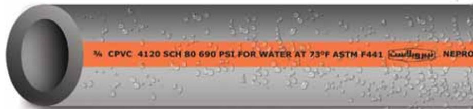
*Manufacturer name, materials designation code, pipe size, schedule size with pressure rating in PSI water at 73°F (23°C) and manufacturing date*
